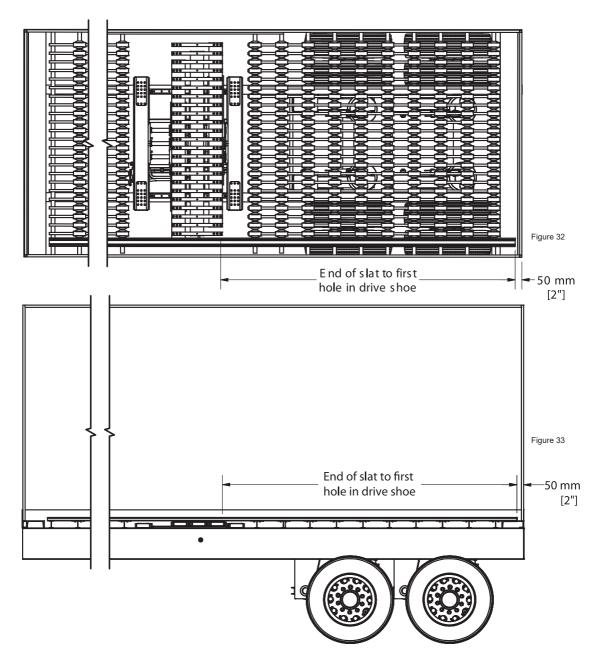
The flooring is to be predrilled before installation. Measure the distance from 50mm inside the door to the first set of holes in the drive shoes. Use this distance to set the shoe drill jig at the first hole. (Note: If multiple trailers are being outfitted with this system, it is beneficial to place the drive units at the same distance from the rear of the trailer, then all the flooring will be drilled in the same location.)
