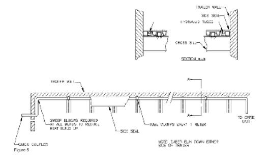
Routing the tubing underneath the cross-members. This option is not recommended, as it can cause problems with truck tire clearance and it makes the tubing very vulnerable.
