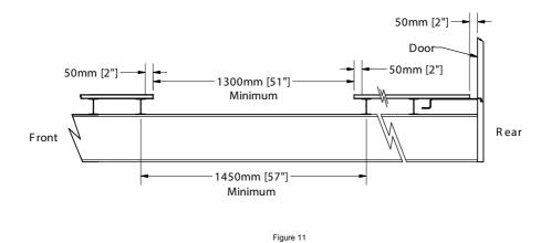
Weld or huck bolt the square tubes to the cross members between the jigs. Move the jigs and make a connection at each intersection of a tube and a cross-member. Welds should be 3mm fillet, 20mm to 30mm long, and centered on the flange. Excessive welding and too little cooling will cause cross-members to warp. Figure 12 suggests a welding pattern. Starting each pass on the same side of the trailer gives sufficient cooling time.
